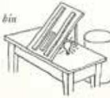
placed on the far side of the table from the artist to catch the film as it drops down from the top end of the channel. The drop should be sufficient to let the wet ink image drawn on the film dry before it hits the bottom of the bin.
