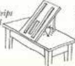
for fixing vertically onto the board about 3 1/2" (90 mm.) apart, thus making a channel on the board above the hole.
