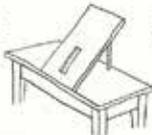
about 2" by 10" (50 mm. x 250 mm.) cut in the board to let light through from behind.
