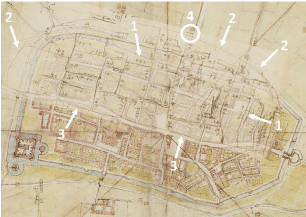
Fig. 7. Overlapping between the sketch of the northern area (cfr. fig. 5) and the map (cfr. Fig. 6) of Imola by Leonardo Da Vinci. Highlighted: 1) the roads inside the built-up area with the annotation of the length; 2) the external perimeter without measures; 3) the Via Emilia traced with a linear course, without taking into account the real irregularities and without measuring the length of its sections; 4) one of the crosses drawn at the external entrance of some roads, hypothetical station points, perhaps to connect different surveying campaigns.
