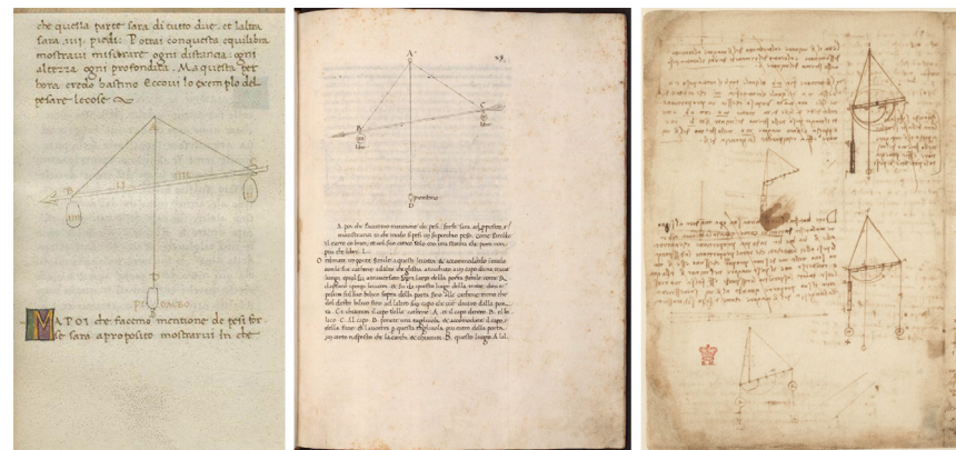
Fig. 3. Drawing of the "Equilibra to measure every weight" in copies of the manuscript (Cambridge and Rouen) and in the Codex Arundel of Leonardo da Vinci.
