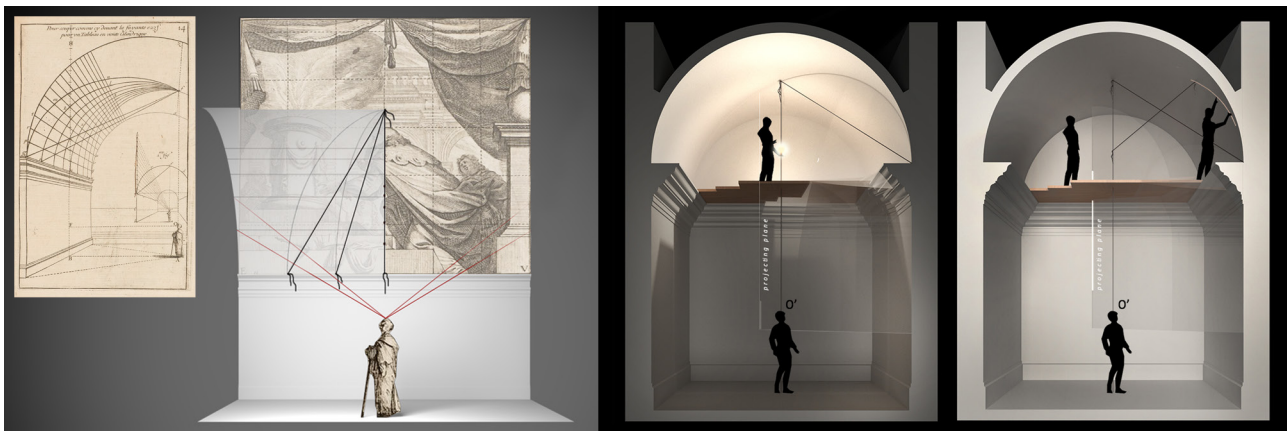
Fig. 8. Abraham Bosse's method for the construction of perspective on irregular surfaces (author's elaboration).
