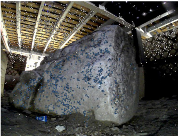
Fig. 7. FSM procedure in inaccessible location: frame of the processing phase and point cloud.
