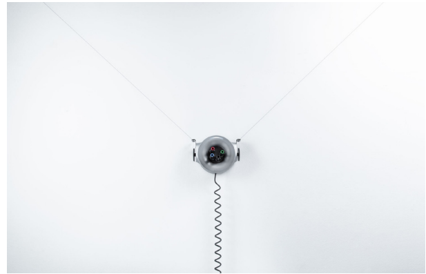
Fig. 8. Scribit (Image credits: Avocado studio). Scribit is a small write&erase robot that can safely draw, cancel and re-draw content on almost any vertical surface, developed by CRA in 2018.
