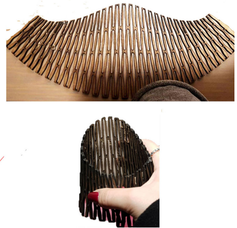
Fig. 3. You can easily manufacture conical and cylindrical surfaces using a "flexible" but not "deformable" material (graphic elaboration by the author).
