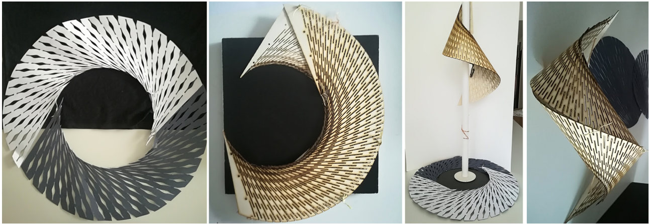
Fig. 12. Prototypes in wood and cardboard for a lamp manufacture: portions of developable helicoids. Design by Mara Capone.
