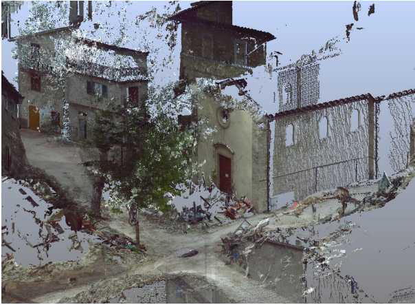
Fig. 2. 3D acquisition of the borough of Grisciano with a Laser Scanner Faro Focus 3D (image by Leonardo Paris).
