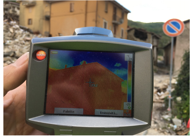
Fig. 3. Data acquisition with thermal imaging camera.
