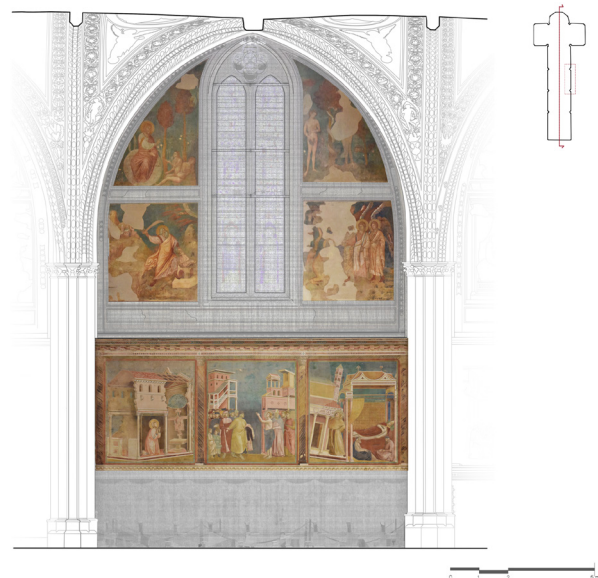
Fig. 2. Example of the digital survey of the Upper Basilica of Assisi, obtained through laser scanning and integrated with photogrammetric data, focusing on one of the bays (graphic elaboration by Roberta Ferretti).
