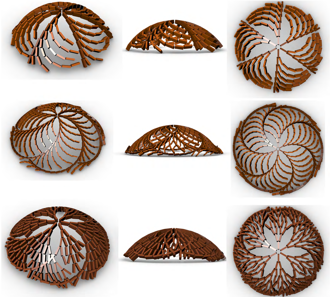
Fig. 6. Computational investigation of the application of organic growth models for structural design in architecture: transposition of biomimetic schemes for the construction of domes through the formal and structural optimisation of the use of brick (elaboration by the authors).
