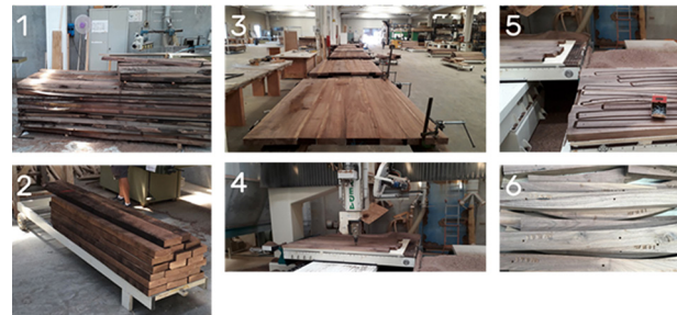
Fig. 6. Stages in the production of panels used to mill the wooden tiles for constructing a physical model of a complex form (photos: Devoto Design).
