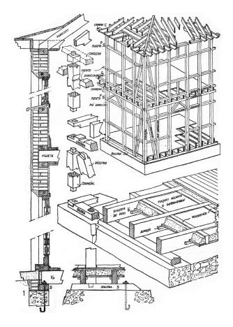
Fig. 8. Construction details of joints and connections on-site (graphic elaboration by the authors).
