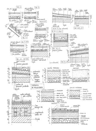
Fig. 10. Construction detail of structural reinforcement (graphic elaboration by the authors).
