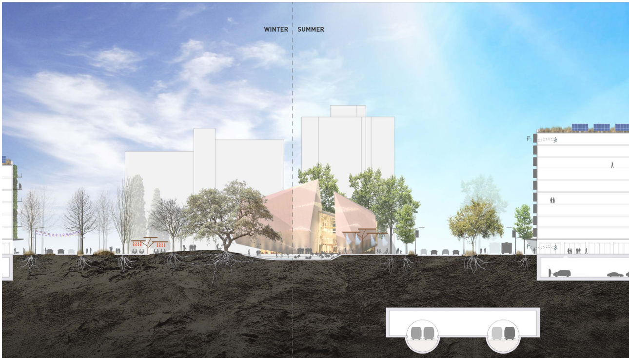
Fig. 6. Madrid Nuevo Norte Landscape Masterplan, Madrid: this section depicts winter and summer, with deciduous trees casting shade on façades in summer. It reveals root systems, often overlooked but crucial to landscape.
