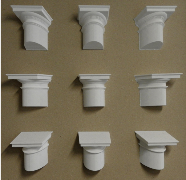
Fig. 12. Composition of one straight and eight oblique capitals, lactic acid polymer (A. Sdegno, 2019).
