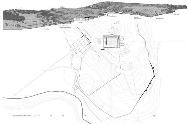
Fig. 8. Upper: 3D model of the central Tiermes area created from the 2x2 km LiDAR laser survey (graphic elaboration by Carlos Rodríguez Fernández from IGN). Bottom: Section and plan of the central area of the Forum and the Roman Baths of Tiermes (graphic elaboration by Carlos Rodríguez Fernández).
