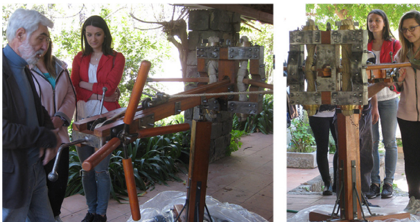
Fig. 1. Scorpione . Prototype reconstructed by F. Russo (2014) on the basis of the modiolus found in Ampurias (Spain); Lab/TAR students (prof. A. Rossi a.y. 2016-2017) visiting the Officine di Archeotecnica .
