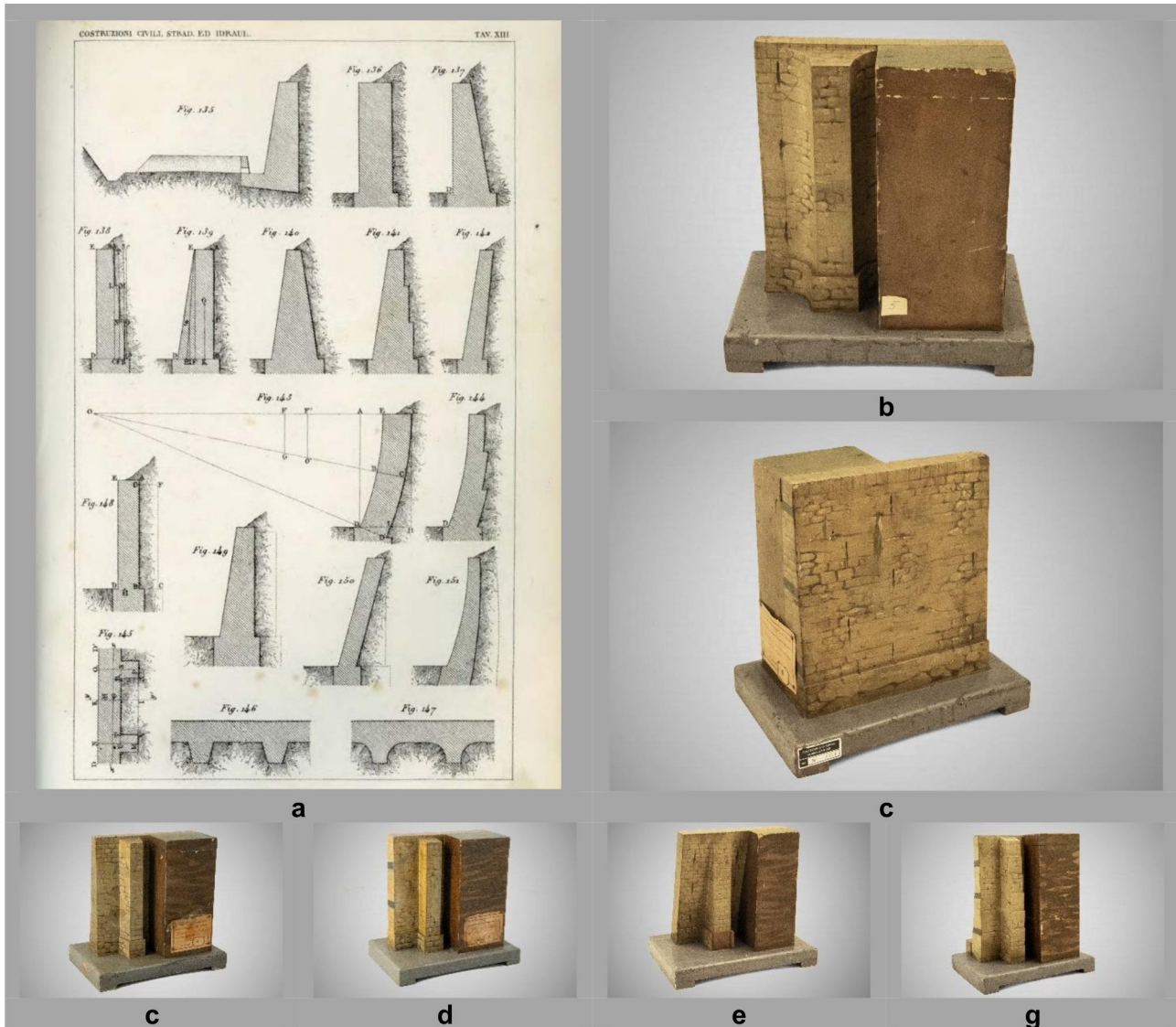
Fig. 1. Retaining walls with internal buttress. a) Curioni 1870. Tav XIII; b-c) model (m. from now on) 5, dim. 240 x 240 x 155 mm; d) m.1, dim. 245 x 250 x 160 mm; e) m.2, dim. 235 x 250 x 160; f) m.3, dim. 255 x 260 x 170; g) m.4, dim. 290 x 250 x 180 (graphic elaboration by M. Pavignano).
