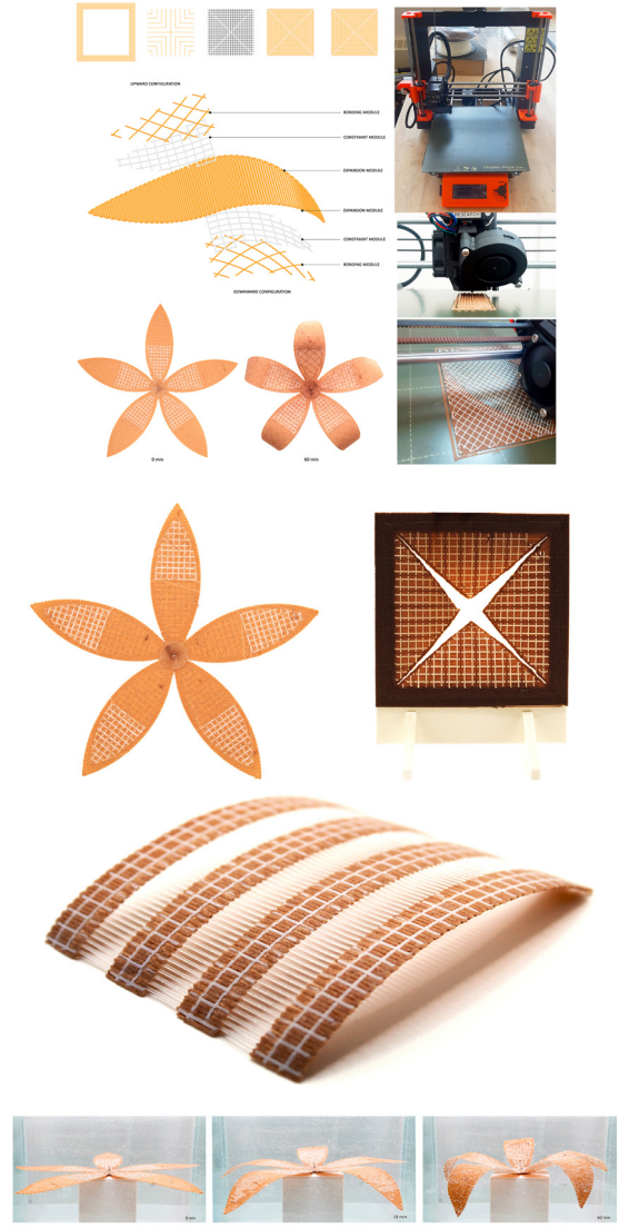
Fig. 12. Execution and installation of the wooden actuators made by additive printing for verification of the hygro-responsivity and kinematics (graphic elaboration by the authors).
