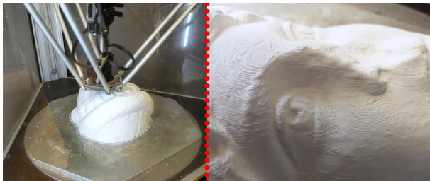
Fig. 4. 3D printing: on the left, the printing process; on the right, detail of the surface: the typical steps of the production process are evident (photo by the author).
