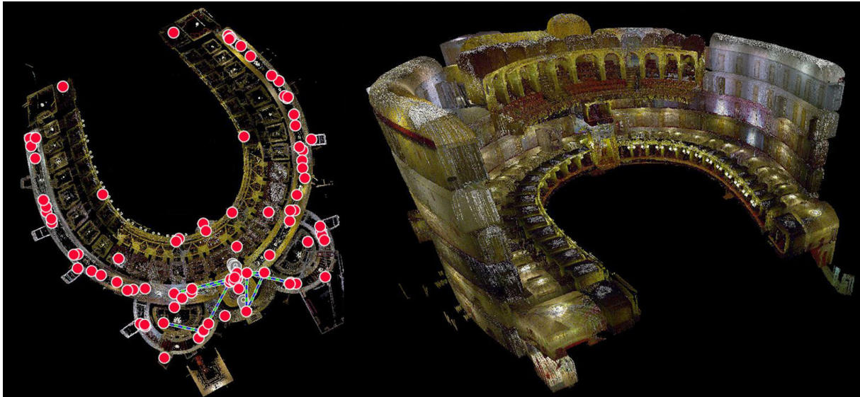
Fig. 5. Point cloud of the Teatro Massimo Bellini in Catania, Italy. Left, draft of the survey taken by Leica Geosystem's P30 terrestrial laser scanner; right, perspective view of the point cloud of the hall (graphic elaborations by the authors).
