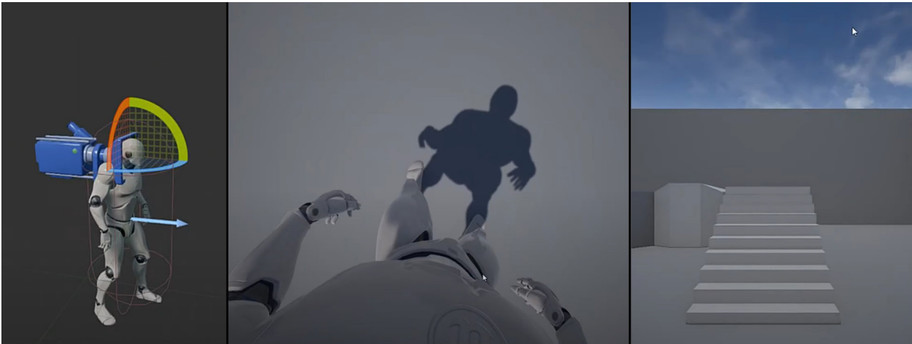
Fig. 2. Rigging of the camera to obtain the first person view (FPV). Unreal 5.
