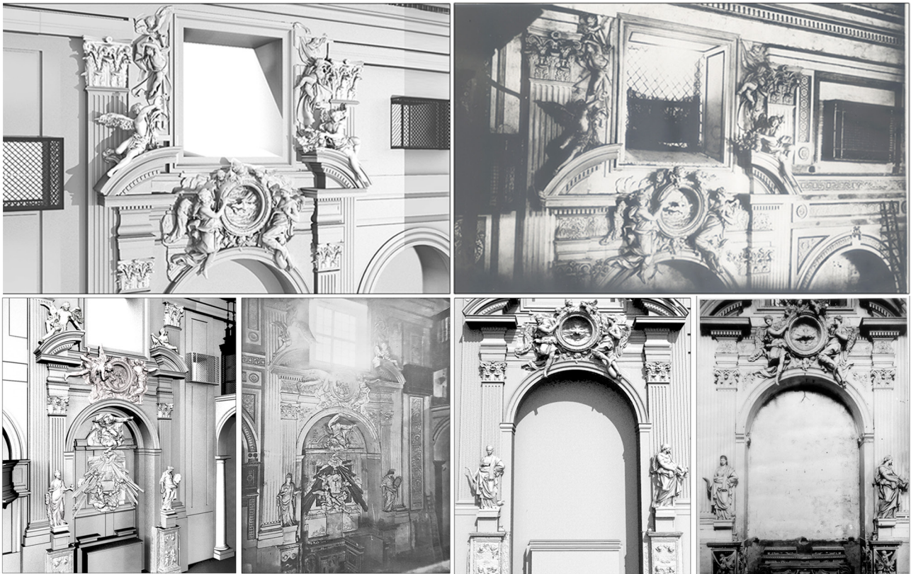
Fig. 7. Visual evaluation of the correspondence between the photographic image of sculptures and their 3D mesh model.
