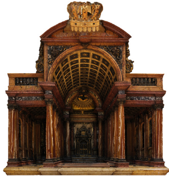
Fig. 8. Tabernacle model from photogrammetric survey, 67-image mosaic processed with SFM software.
