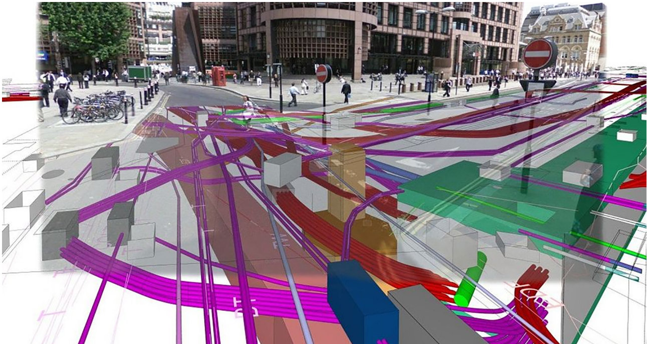
Fig. 15. Use of BIM for urban-scale designs of technical systems.
