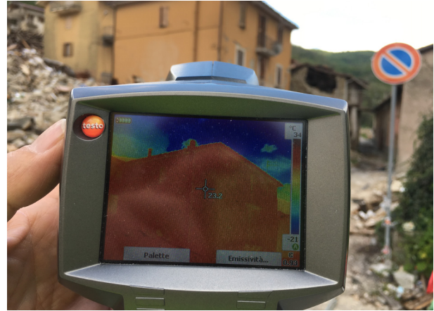
Fig. 3. Data acquisition with thermal imaging camera.
